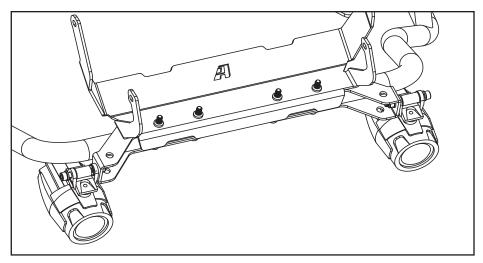
Repeat on the left side. Use 5mm allen tool and 10mm spanner to tighten each light mount screw to 8 Nm.
