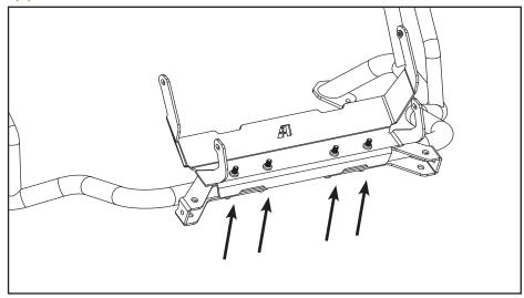
2 Place the AltRider light mount brackets around the tube, and sandwich them to the under-nose bracket. Install the M6 x 50mm socket cap screws with washers. Torque to 8.7 Nm.
