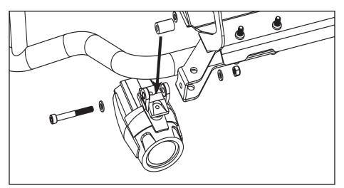
Place the aluminum spacer between the light mount yoke. Use thin nylon washers (may not be needed) to ensure a snug fit. Insert the M6 x 50mm screw and washer, and use another washer and the nylon insert locknut on the inner side of the bracket.
