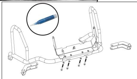
Use 5mm allen tool and remove M6 socket cap screws that hold the bars to the main under-nose bracket. Get ready the two light mount brackets, four M6x50mm screws, and four M6 washers. Add a drop of thread locker to each screw.
